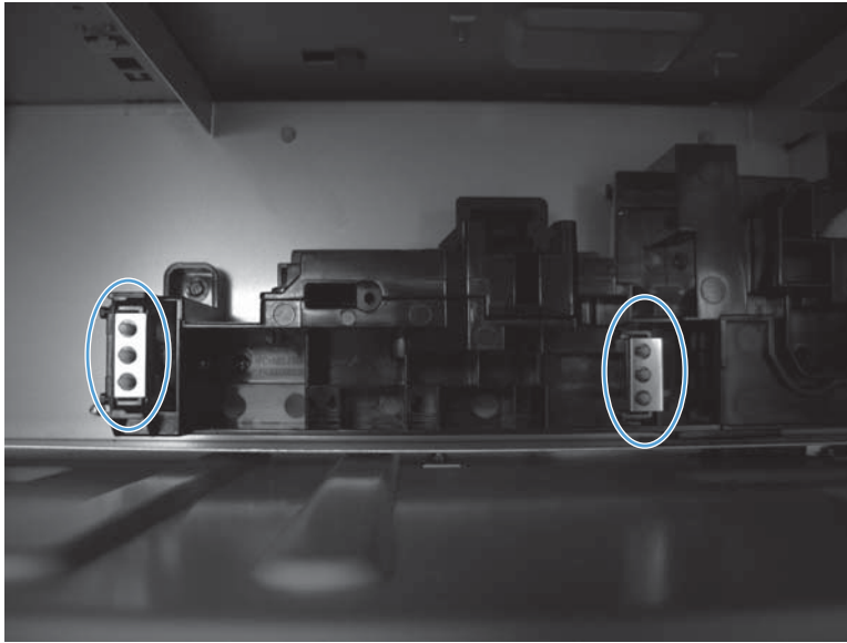
Figure 2-21 Tray 4 paper size switches
